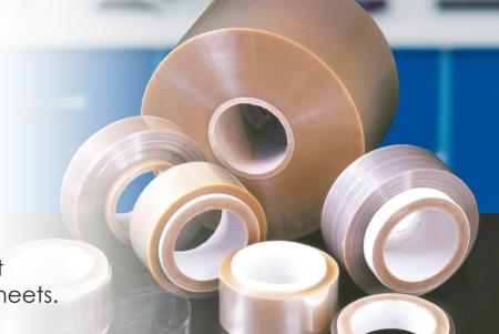
MEMBRA-CEL® dialysis membranes are made of regenerated cellulose using the viscose process. These semi-permeable membranes have distinct Molecular Weight Cut-Off (MWCOs) of 14,000, 7,000 and 3,500 daltons by excluding macromolecules with molecular radii from 50 down to 35 angstroms.
